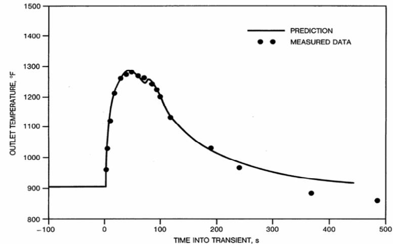
Unprotected Loss-of-flow Test
