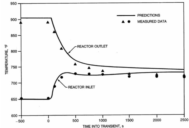
Unprotected Loss-of-heat-sink Test
